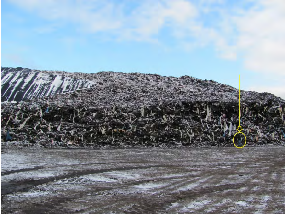
Figure 3: 80,000-ton Pile of Post-Consumer Shingles
